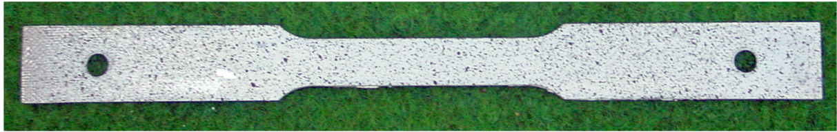
Fig. 3. The surface preparation of the specimens for non-contact optical deformation measurements
