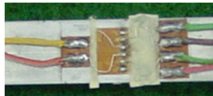
Fig. 2. Arrangement of a strain gauge rosette on the specimen
