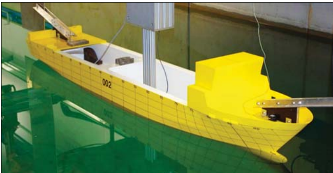
Fig. 3. Model of the case study vessel N21 in towing tank
