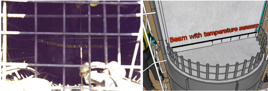
Fig. 4. The beam with the PT100 type temperature sensors located inside the column
