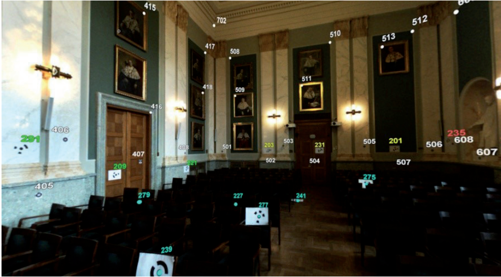
Fig. 2. Natural and signaled (coded and uncoded) targets in the assembly hall Source: http://kwiatek.krakow.pl/3D_modelling_from_immersive_video/aula_agh
