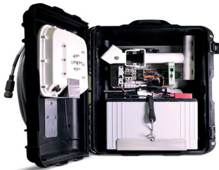
Fig. 1. Radar traffic detector Wavetronix's Portable SmartSensor HD Radar [12]
