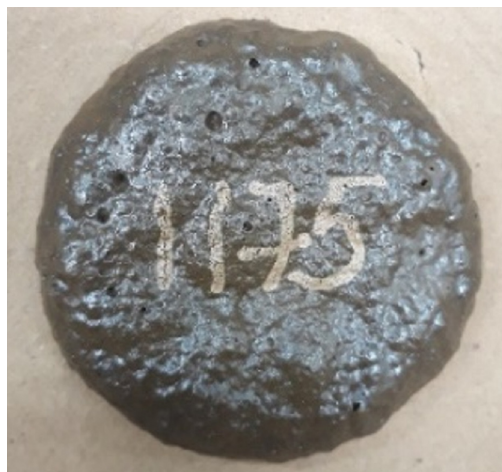
Fig. 1. Thin fly ash geopolymers heated beyond 1150^\circ\text{C}
