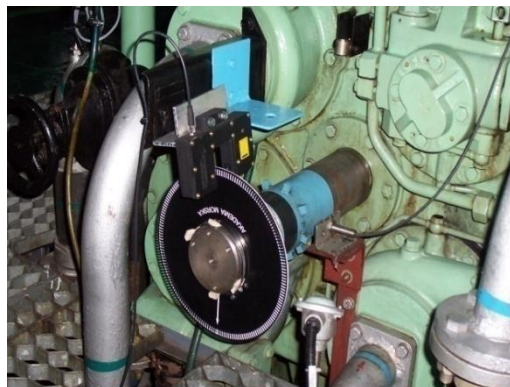
Fig. 2. Encoder disc and sensor mounted at the crankshaft
