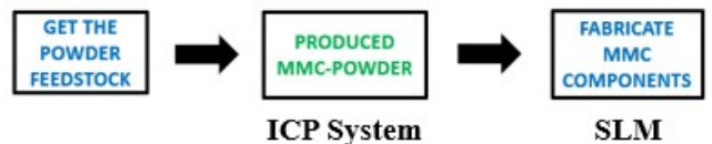
Fig. 5. The inductively coupled plasma approach for in-situ MMC material development
