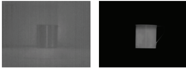
Fig. 1. Poor contrast (left) and good contrast (right) IR images. Left: mug of water, temp. about 22°C, right: mug of water, temp. about 35°C
