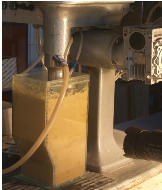
Fig. 1. Non-overflowing glass cell used to determine the maximum froth depth
