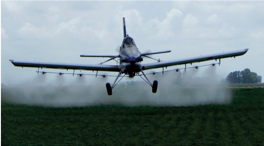
Fig. 9. The aircraft equipped with a similar sprayer to the one used in this work with the central pump propelled by an external flow axial turbine, omitted in the computational geometry [13]
