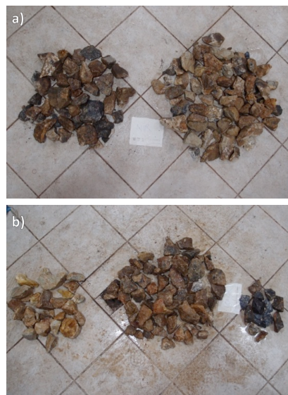
Fig. 11. Products after separation a) NIR sorting b) Color sorting
