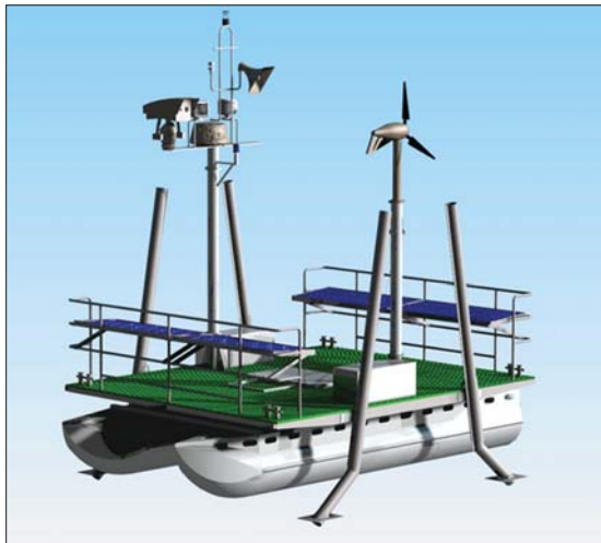
Fig. 3. Observation platform with a transport catamaran
