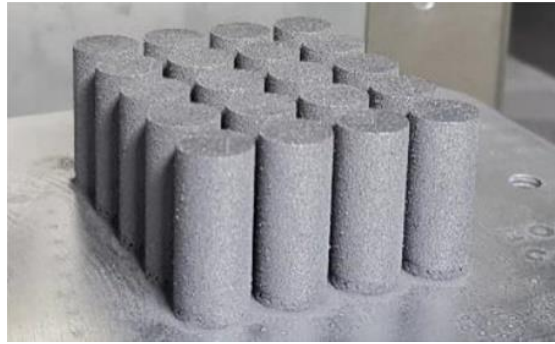
Fig. 2. 316L alloy specimens manufactured via SLM technology.
