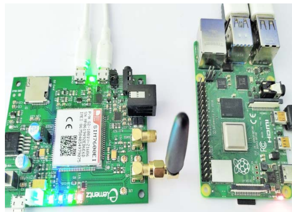
Fig. 4. The SIM7600 GSM GPS 4G LTE module with the Raspberry Pi
