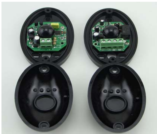
Fig. 3. The ABO-20 single beam IR sensor
