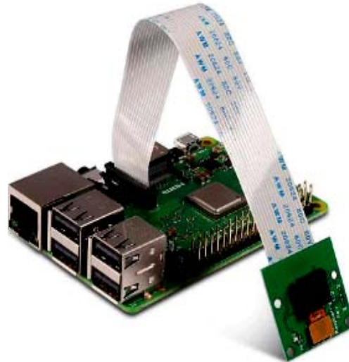
Fig. 5. The Pi Camera connected to the Raspberry Pi
