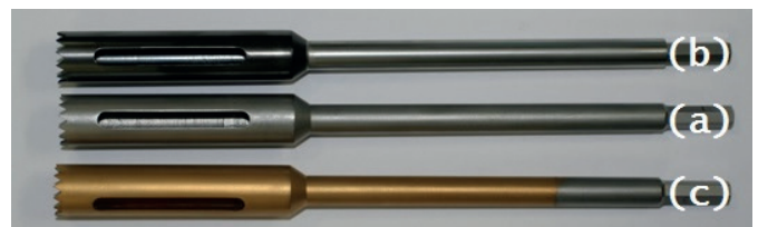
Fig. 2. Surgical drill bits for field tests: (a) no surface modification, (b) DLC, (c) TiN
