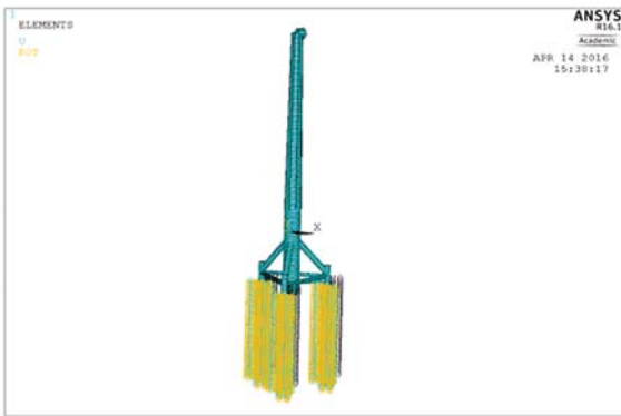
Fig. 2. FE model of the tripod
