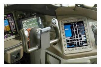
Figure 3. Integrated "electronic flight bag" (Jeppesen, 2012)
