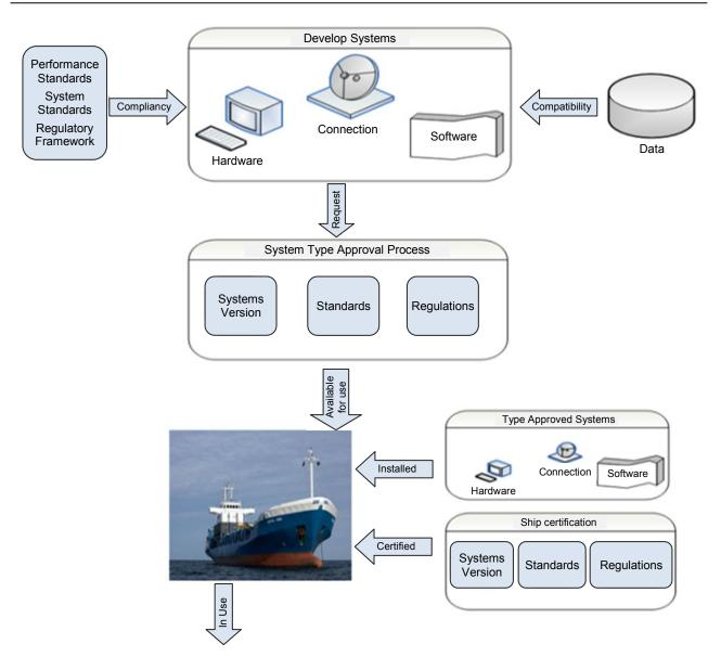
Figure 2. Current type approval process (Bergmann, 2015)
