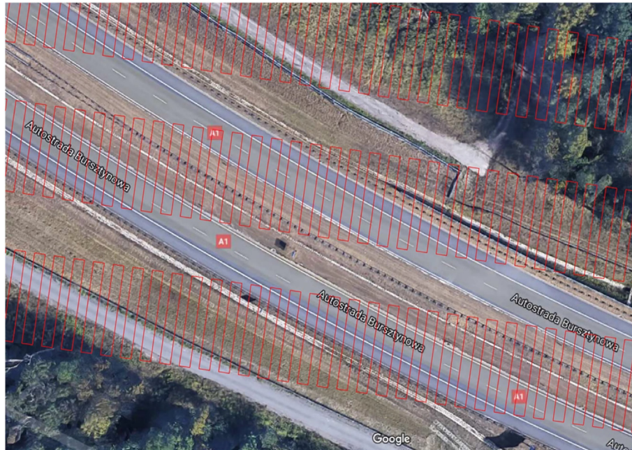
Fig. 7. Sample arrangement of pixels in the analysed section of motorway A1 Bytom (Poland).
