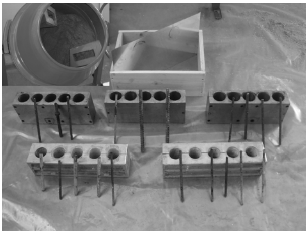
Fig. 7a. Moulds with two different shapes, cylindrical and triangular.
