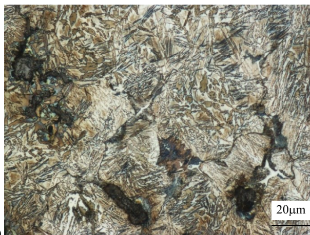
b) microstructure: compacted graphite, ausferrite, carbides, pearlite
