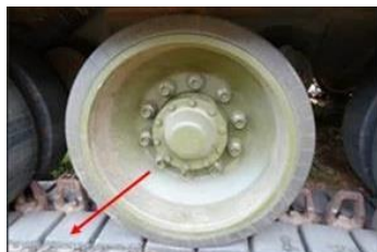
Fig. 7. Rubber cushions on the inner surface of the links of crawler tracks
