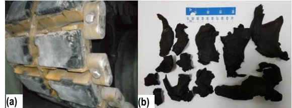
Fig. 8. Rubber cover plates: (a) with varying degree of wear and tear and (b) torn out rubber pad fragments
