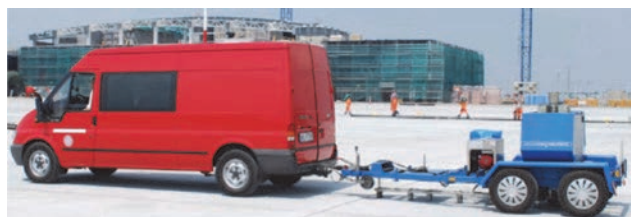
Fig. 3. Device intended for measuring the rebound deflections of airport pavements
