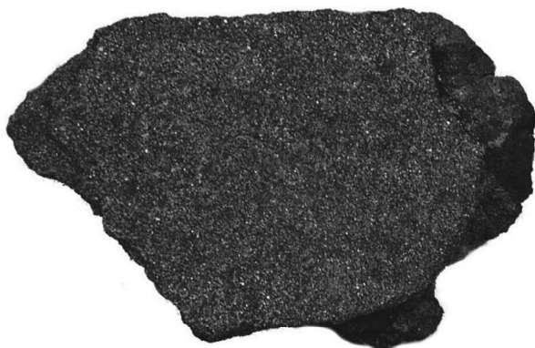
Fig. 9. Photography of oil sand extracted from the Asphalt Ridge deposit in Vernal (Utah, USA), source: www.ostseis.anl.gov/guide/photos/index.cfm
