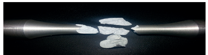
Fig. 6. Parts of aluminium alloy specimens after losing the coherence - temperature of 560 °C.
