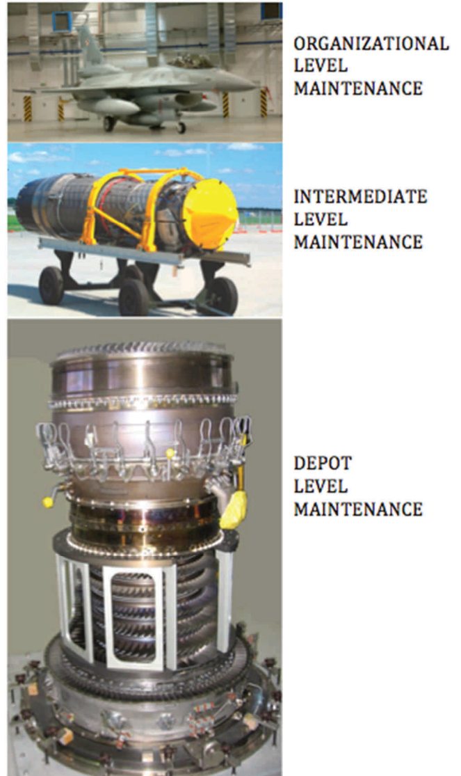
Fig. 3. Levels of maintenance
