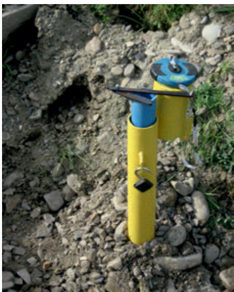
Rys. 14 Pomiar osiadań Fig. 14 The subsidence measurements
