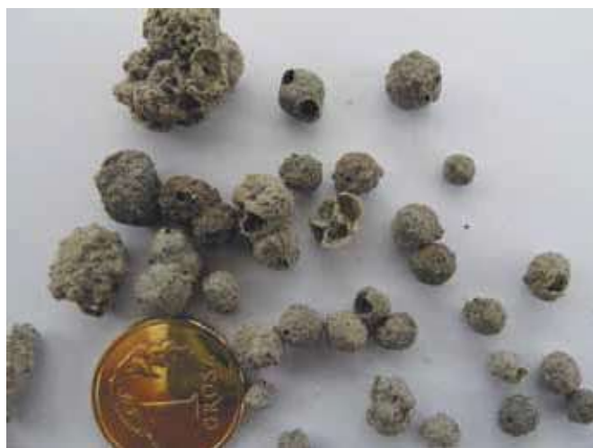
Rys. 2. Konglomeraty mikrosferowe. Fig. 2. Conglomerates of cenospheres
