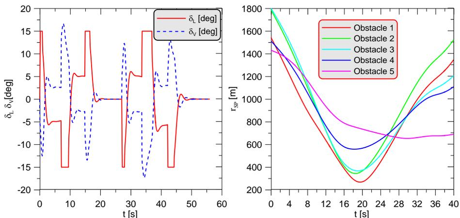
Fig. 5a, 5b. Ailerons and rudder deflections and airplane — to-obstacle distance (flaps deflected) [own work]
