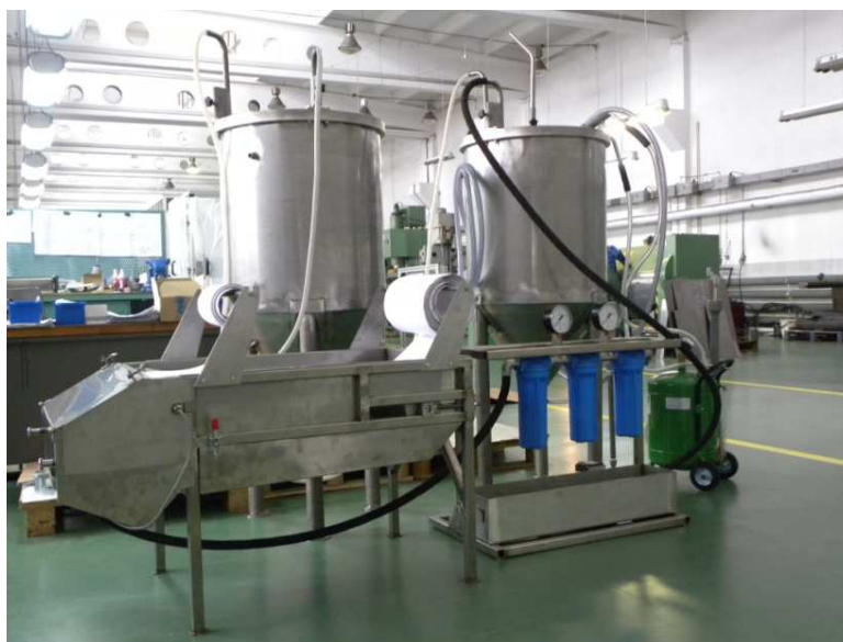
Fig. 2. A device for the recycling of waste cutting fluid
