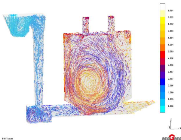
Fig. 5. Fill Tracer simulation for the second simulation with respect to aging time (in seconds)
