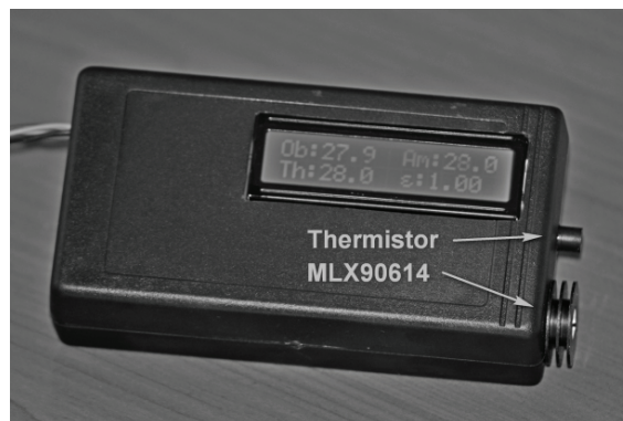
Fig. 4. Developed device for emissivity estimation
