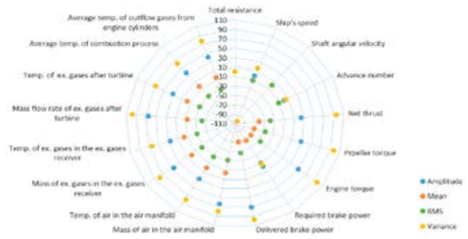
Fig. 13. Relative changes in the statistical parameters of the system variables (in percentages) under propeller ventilation
