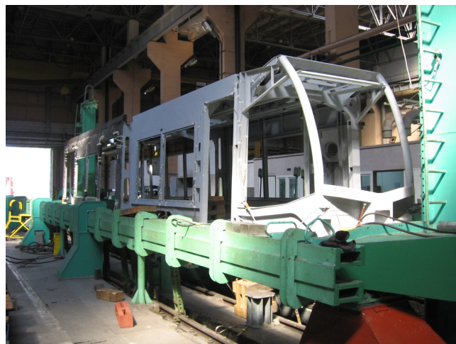
Fig. 2. View of the construction of the tram body during static strength tests
