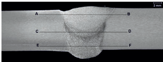
Fig. 2. Macroscopic cross-section of a specimen made of AW7020 alloy welded with deposited metal 1, with marked lines of subsequent hardness penetration patterns and results of the HV5 hardness measurements performed along those lines at the joint cross-section
