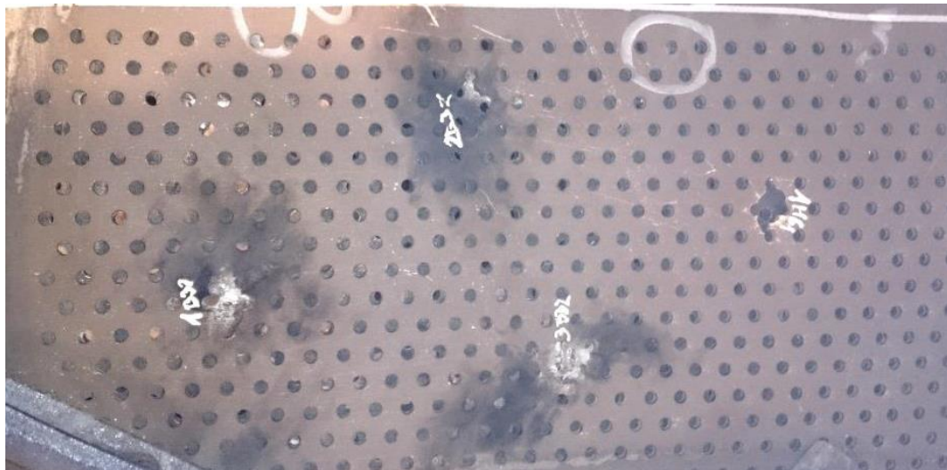
Rys. 5. Fotografia układu blach perforowanych 3mm+8mm po ostrzale pociskiem kal. 7,62x54 mm R API B-32 Figure 5. Photograph of a combination of perforated plates 3mm+8mm after firing by the round R API B-32 of 7.62x54 mm calibre
