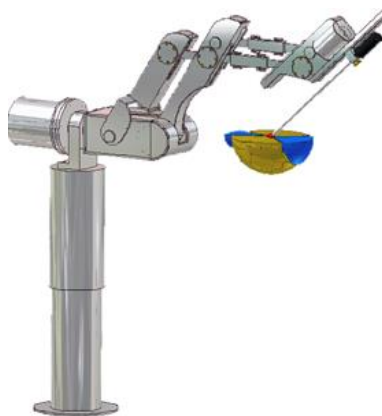
Fig. 2. Virtual prototype of the medical robot with possibility to change access port
