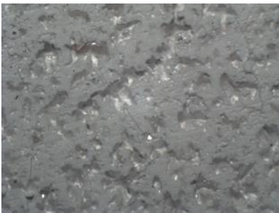
Fig. 11. Ceramic mould after 8-hour annealing at a temperature of 1100°C (magnification 30x)
