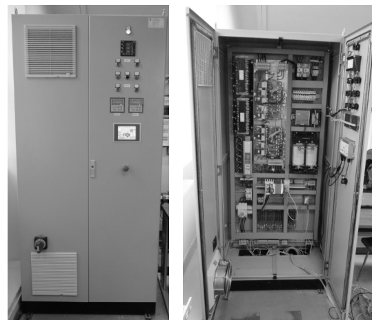
Fig. 4. Ready PEU of 30kW power (manufactured by Power Electronics Company "Twerd")
