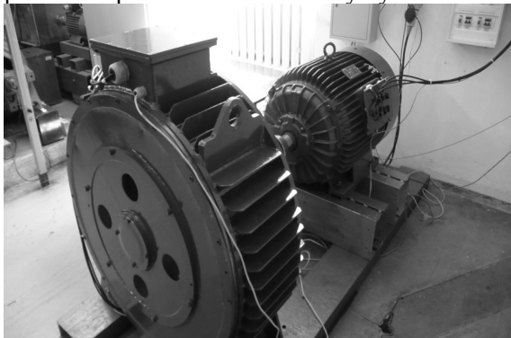
Fig. 2. Laboratory hydro-set of 30kW
