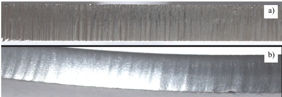
Fig. 2. Macroscopic view of the steel after cutting process: a) by laser; b) by plasma arc
