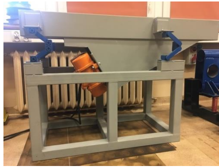
Figure 6. Photograph of the research stand. The suspension system based on AB 15 vibroinsulators
