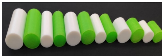
Fig. 5. Samples made by CNC machining and 3D printing technology
