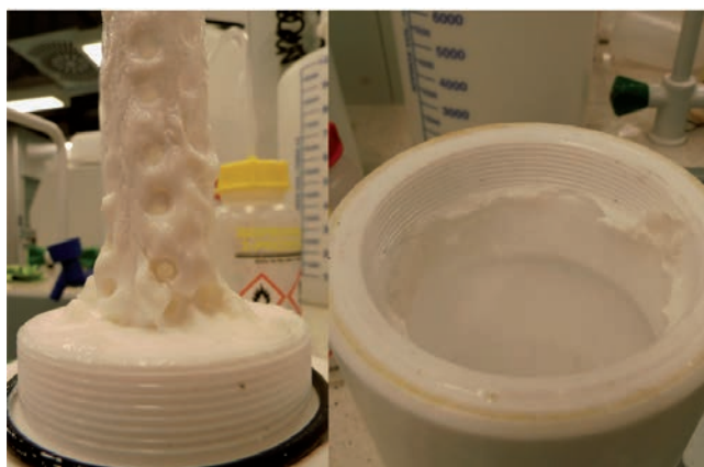
Fig. 3. Hydroxyapatite deposited on the damper during stop-flow reactions Source: IHPP PAS.
