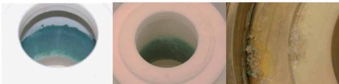
Fig. 4. Cobalt doped ZnO NPs embedded in the reaction chamber during a few stop-flow reactions Source: IHPP PAS.
