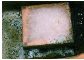
Fig. 11. ERAWA-1 cassette after combustion of napalm on it and around it
