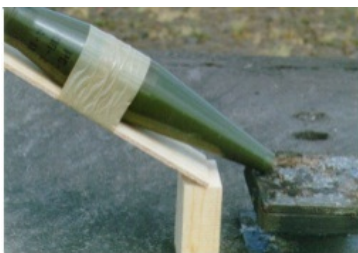
Fig. 10. Test of ERAWA-1 cassette resistance to detonation and destruction during burning napalm on it and around it
