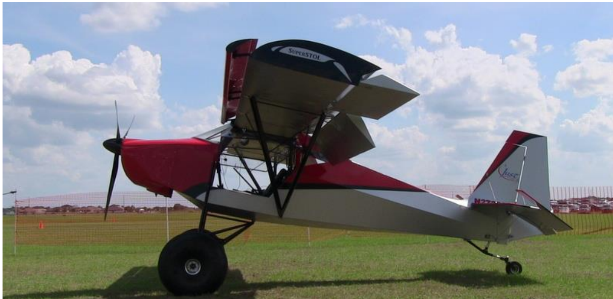
Fig. 1. Wing mechanization on a high-performance Just Aircraft Super STOL airplane (note the low-pressure tundra tyres with a big diameter)
