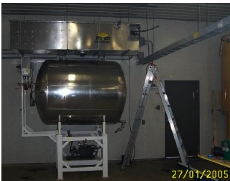
Fig. 3. Honey concentrator operating at French Bee Farm [16].
