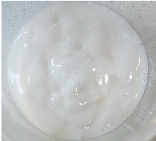
Fig. 7. The UnderDril mud weighted with calcium carbonate bridging agent
