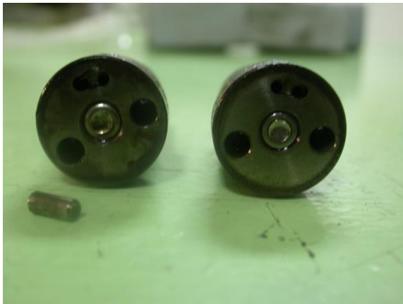
Fig. 15. Broken needle shafts of injector nozzles
