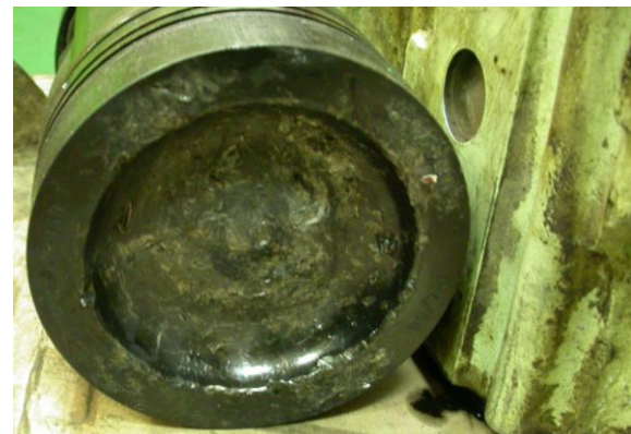
Fig. 8. The piston failure
