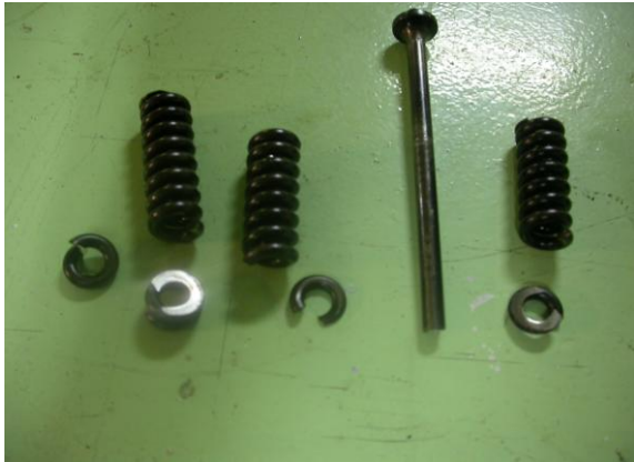
Fig. 14. Broken springs and damaged push rod of fuel injectors
