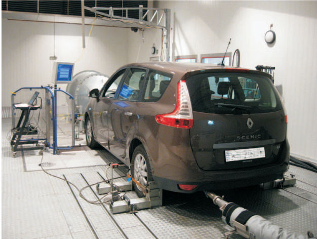
Fig. 4. Interior view of BOSMAL's exhaust emission laboratory, showing a vehicle mounted on the chassis dynamometer, together with the driver's aid (monitor) and the windspeed fan, all within the climatic chamber ( -35\text{ }^\circ\text{C} to +60\text{ }^\circ\text{C} )
