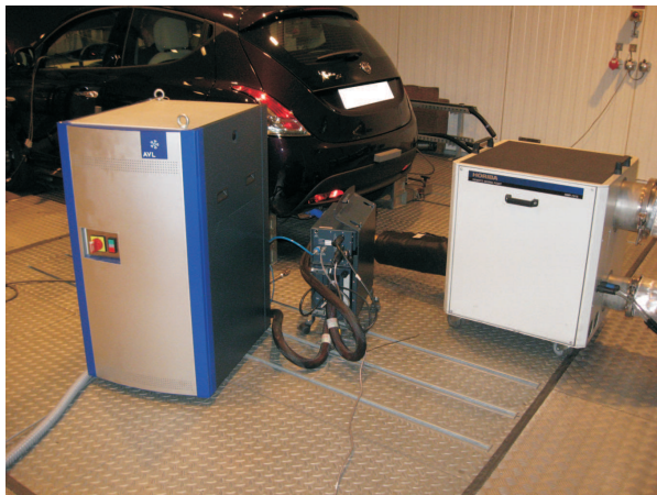
Fig. 5. A specialized automotive emissions analyser for measuring concentrations of \text{NH}_3 in the exhaust gas of multiple vehicle types
