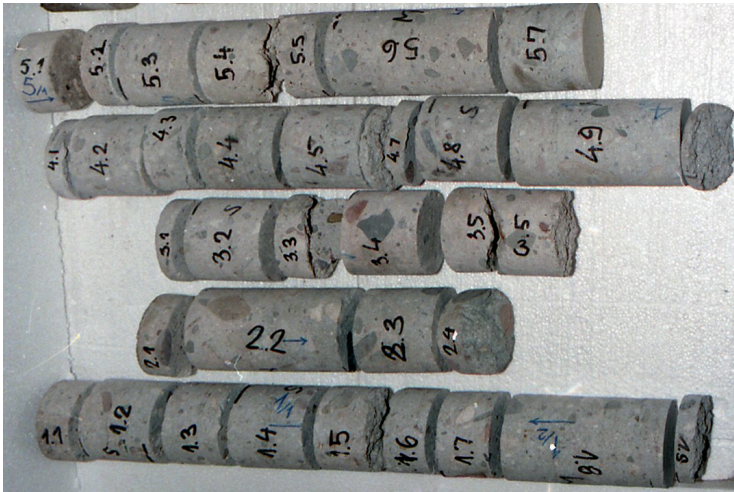
Fig. 4. The cores from the bottom plate of the foundation no. 1 cut into samples
